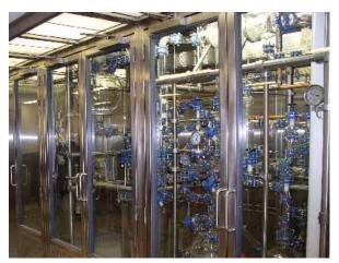
These modular enclosures can be provided with either horizontal flow or vertical downflow systems depending upon the application. Localised flow can also be provided both inside and outside the enclosure to ensure the added protection of the operator during the loading process.
