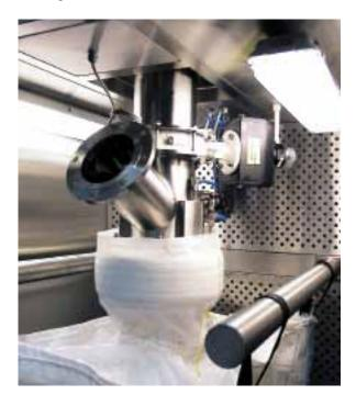
To complement our range of Pack-off heads, Howorth are able to offer a variety of secondary pack-off containment products in the form of booths and isolators. By utilising a secondary containment solution, operator protection can be improved and containment levels of less than  $1 \mu g/m^3$  can be achieved.
