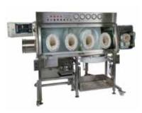
The safe handling of bulk chemicals and potent pharmaceutical compounds demands an environment which provides uncompromising total barrier isolation.
