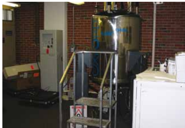
A shot of the Varian Inova 600MHz NMR spectrometer with the N2 generator in the background
