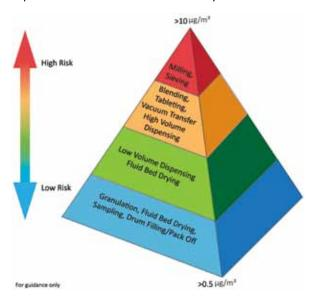
Independent testing of Howorth's 4D High Containment Screen has confirmed that OELs as low as  $0.5\mu g/m^3$  can be achieved when operated in conjunction with agreed SOPs. Processes considered to have a higher risk of exposure also benefit from a considerable reduction in OELs.
